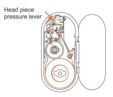
• Close the paper roll press block, tighten the paper winding shaft, screw the head piece pressure lever, close the side cover of printer, then long press FEED button to roll the paper
